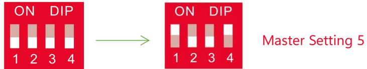
the DIP switch of slaves need to turn the "#4" to "ON" at the same time while the master is setting 5.
