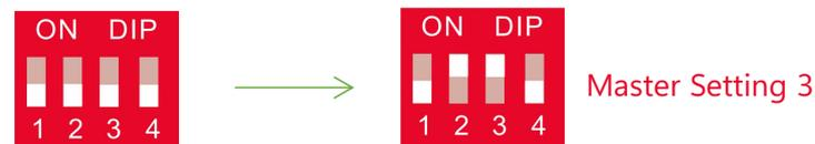
5. If the battery communicates with the Schneider Conext Series, turn the master DIP switch "#1" and "#3" to "ON".
