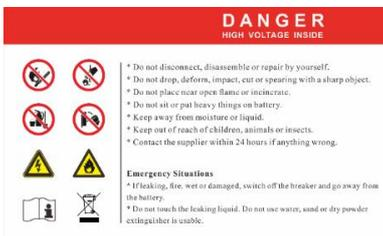
Dangerous goods warning label on the top of the battery module
